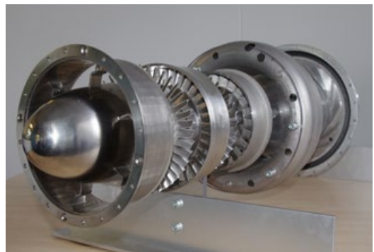
3D print of a small jet engine. Image: Monash University
