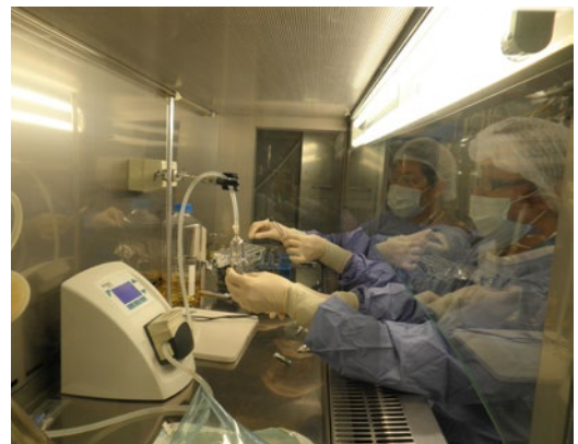
CSIRO Recombinant Protein Production Facility (RPPF) staff using sterile microbiological medium under simulated manufacturing conditions, to validate aseptic procedures.
