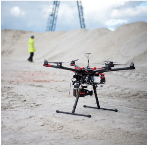
The Hovermap drone payload can fly autonomously in GPS-denied environments to create 3-D maps.
