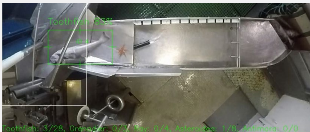
Automated species identification and counting of freshly caught fish on a boat. Credit: Austral Fisheries.
