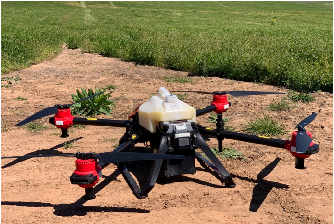
This XAg P30 spray drone with capacity of 16 litres is being used to apply different chemical and bio-fungicidal treatments to cropping trials at the Boorowa Agricultural Research Station.
